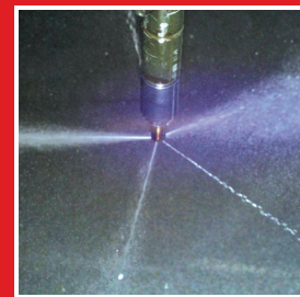
Poor spray pattern with clogged injector.
